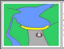
**Temporary cofferdam** with diversion channel: **Superior Dam**<sup>™</sup> replaces earthen or rock cofferdams, sheet piling, and sand bags. Route water around in-stream construction projects. Quick to install, easy to remove, and truly reusable many times. No fill is added to the waterway, and should the water level rise and overtop the dam, it will stay in place.
